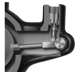
Simple Lever Seat Detail
